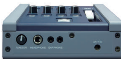
Type A : CB-186-S 2ch monitor, with fader
